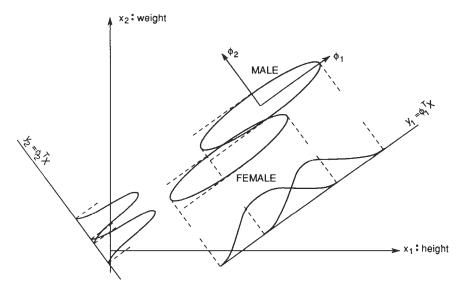
Fig. 10-1 An example of feature extraction for classification.
