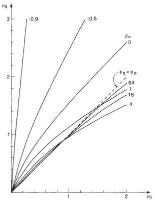
Fig. 3-19 Relation between  $\mu_0$  and  $\mu_g$  for gamma densities.
