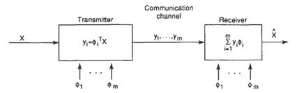
Fig. 9-4 Data compression in communication.
