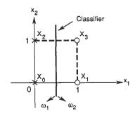
Fig. 8-1 Linearly separable example.
