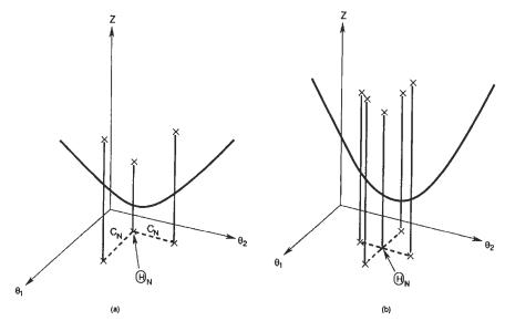
Fig. 8-6 Minimum-point-finding problem for a multivariate case.
