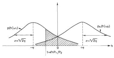
Fig. 3-15 Density functions of h(X) for normal distributions with equal covariances.
