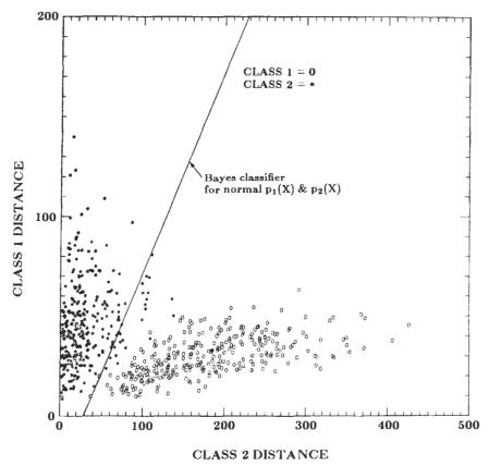
Fig. 4-9  $d^2$ -display of a radar data.
