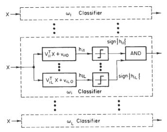
Fig. 4-13 Implementation of a piecewise linear classifier.
