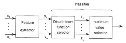
Fig. 10-4 Structure of a classifier.
