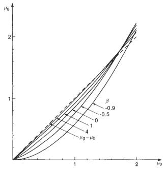
**Fig. 3-21** Relation between  $\mu_0$  and  $\mu_g$  after log transformation.
