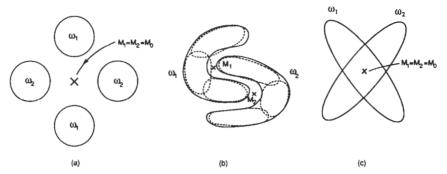
**Fig. 10-5** Examples for which  $tr(S_w^{-1}S_h)$  does not work.
