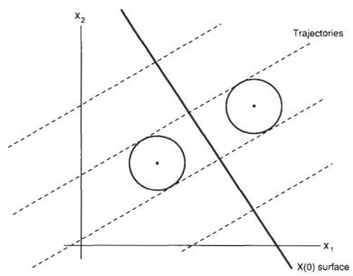
Fig. 10-15 Hypersurface and trajectories for features with  $\lambda_1 = 1$ .
