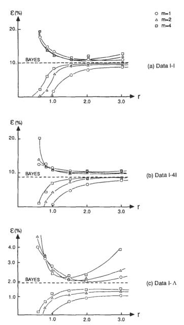
Fig. 7-12 Effect of kernel shape on Parzen classification.
