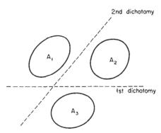
Fig. 11-2 Multiple dichotomy of three classes of samples.
