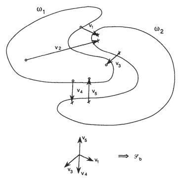
Fig. 10-6 Nonparametric between-class scatter.
