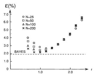
Fig. 7-8 Effect of sample size on Parzen classification.
