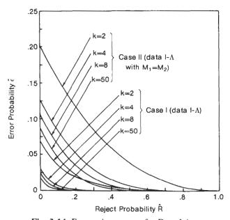
Fig. 3-14 Error-reject curves for Data *I*-Λ.
