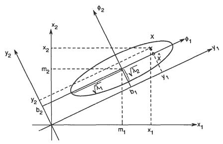
Fig. 9-2 A two-dimensional example of the Karhunen-Loéve expansion.
