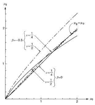
Fig. 3-20 Relation between  $\mu_0$  and  $\mu_g$  after transformation.
