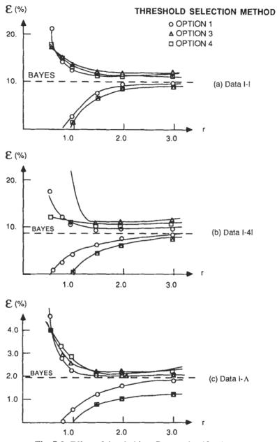
Fig. 7-9 Effect of threshold on Parzen classification.
