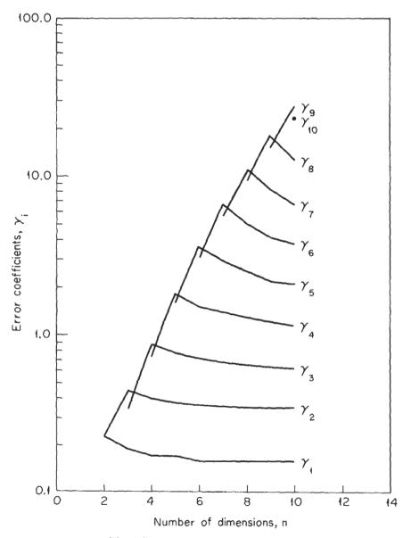
Fig. 9-7 Error coefficients for  $\rho = 0.1$ .
