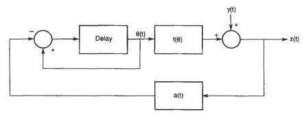
Fig. 8-4 Equivalent feedback circuit.
