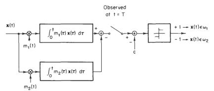
Fig. 4-1 Block diagram of a correlation classifier.
