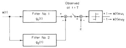
Fig. 4-3 Block diagram of a matched filter classifier.
