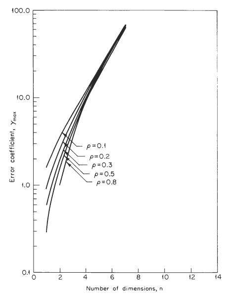
Fig. 9-8 Value of the maximum error coefficient.
